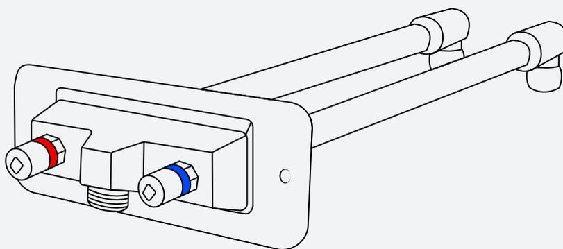
Example of outdoor tap with quick release adapter installed:
